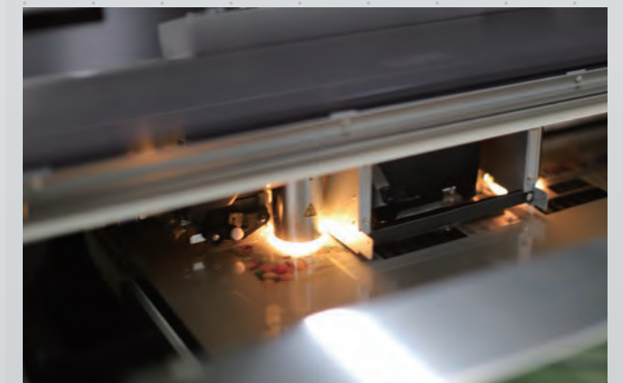
Equipped with a heater for ink adhesion to the printer head.
